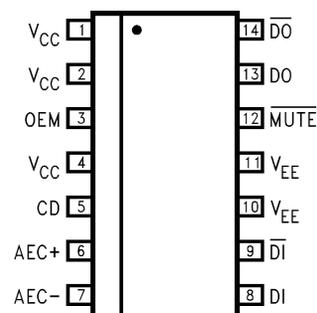
Figure 1. 14-Pin SOIC (Top View)
