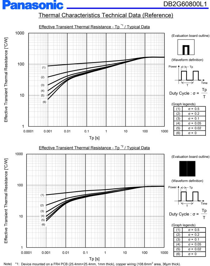
\*2: Device mounted on a FR4 PCB (25.4mm×25.4mm, 1mm thick), copper wiring (620.0mm<sup>2</sup> area, 36µm thick).
