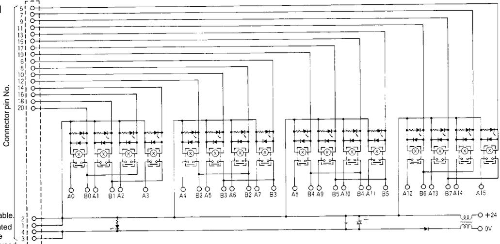
Note: Wiring shown above is for G6D Power Relays.
