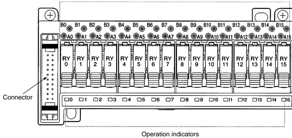
Note: When the terminal block and relay block are connected to each other, each electrical check terminal of the relay block is connected to the corresponding terminal of the terminal block.
