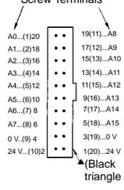
Connector pin numbers in parentheses are for G79 Cable.
