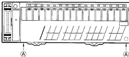
Use the Relay Removal Tool provided to the left of the screw terminals when replacing relays.
