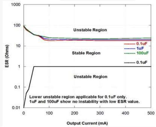
Figure 12. Output Stability vs. Output Capacitor Change
