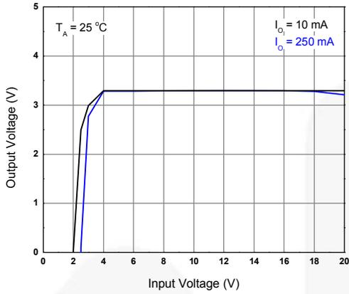
Figure 9. Output Voltage vs. Input Voltage
