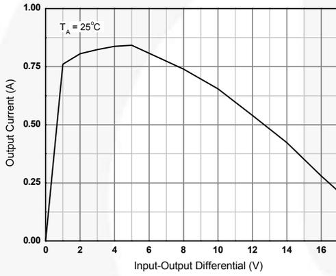
**Figure 5. Peak Output Current**
