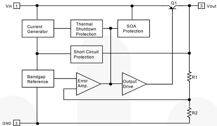
Figure 1. Block Diagram
