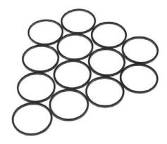
Description: These plastic shaft spacers have an inner diameter of 1" and a thickness of 1/16". These spacers are ideal for spacing out an area between a bearing and a shaft collar to reduce metal to metal contact.
