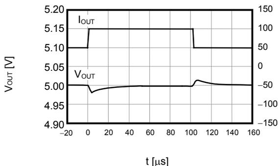
**(3) ON/OFF pin transient response characteristics**
