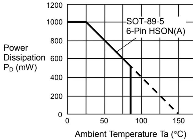
Figure 4 Power Dissipation of Package (Mounted on Printed Circuit Board)
