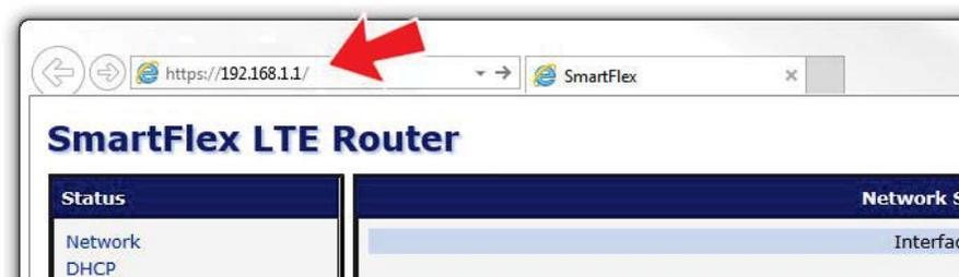
Figure 50: Entering the IP address of the router
