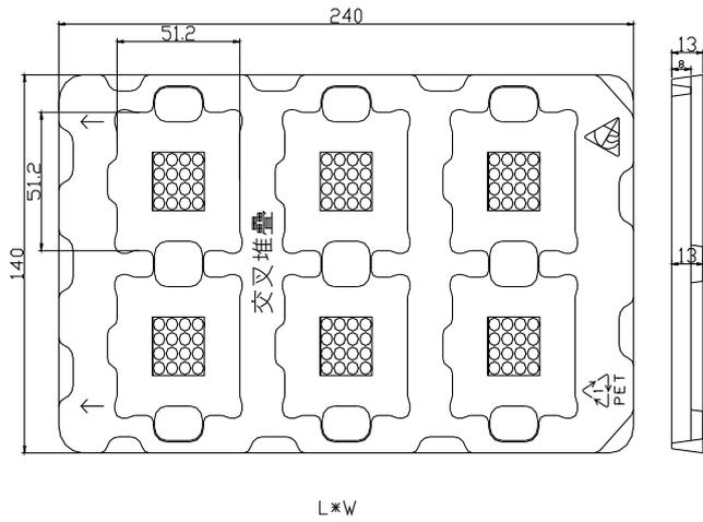
Fig. 5 - 6 Pieces LED Array in One Tray
