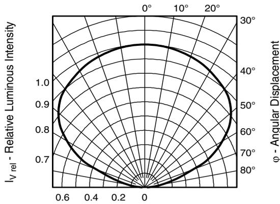
Fig. 2 - Relative Intensity vs. Angular Displacement
